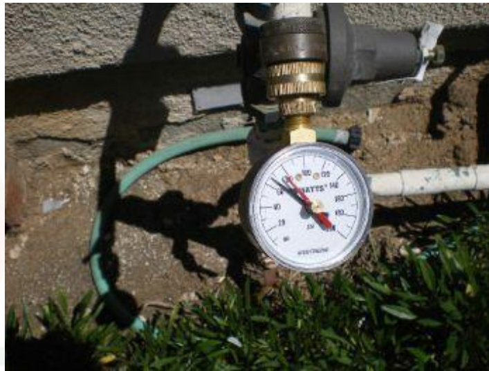
Water Pressure Gauge reading approximately 70 PSI
